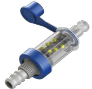
Part 601 116-TH Single Port 10mm [3/8"] Hose With external thread M16x1.5
